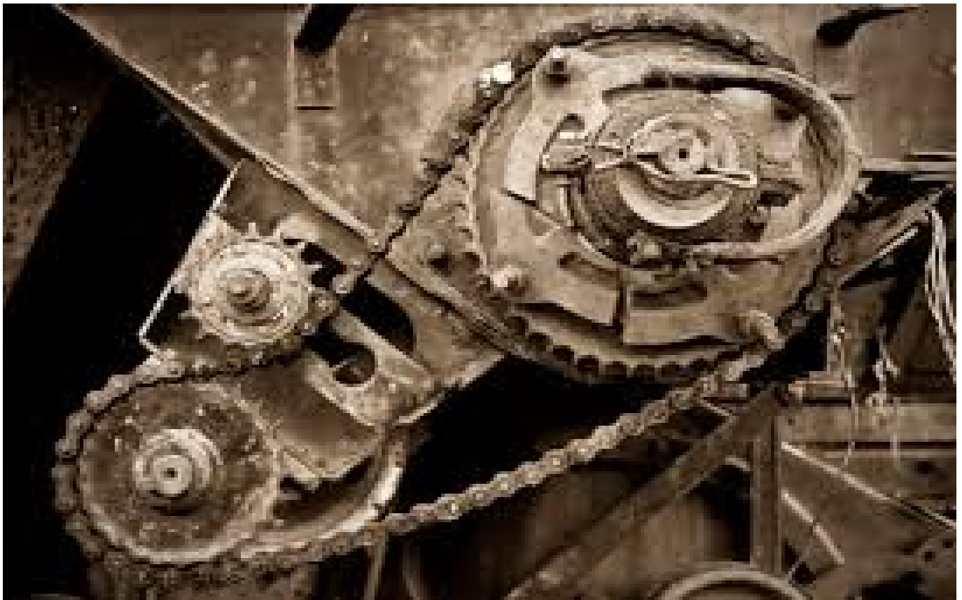
Image #7 - Are exposed belts, chains, and spinning parts less than 7 feet from the flo...
